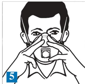
5. Using both hands, mould noseclip to the shape of the lower part of the nose. DO NOT pinch the nosepiece using only one hand as this may result in less effective respirator performance.
