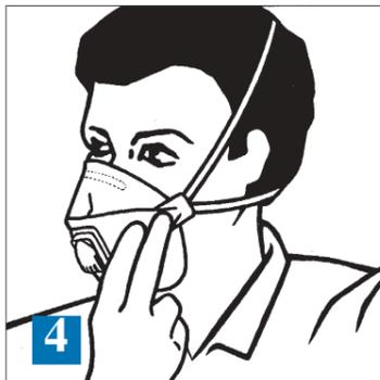
4. Locate the lower strap below the ears and the upper strap across the crown of the head. Adjust top and bottom panels for a comfortable fit.
